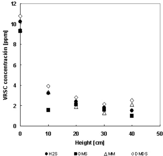
Fig. 7 VRSC concentration (ppm) vs. biofilter height (cm).
