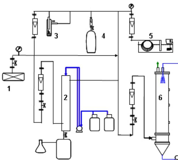
**Fig. 1 Experimental system for the oxidation of sulphur compounds in biotrickling filter.** (1) Compressor; (2)  $H_2S$  Generator; (3) Generator DMDS; (4) Cylinder MM; (5) DMDS Generator; (6) Biotrickling filter.
