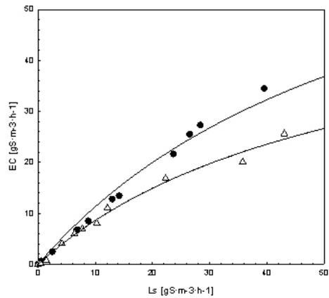
Fig. 5 Elimination capacity (EC) vs Load of sulphur (Ls) in biofilter inoculated with *T. thiooparus* for H<sub>2</sub>S (●) and MM (Δ).
