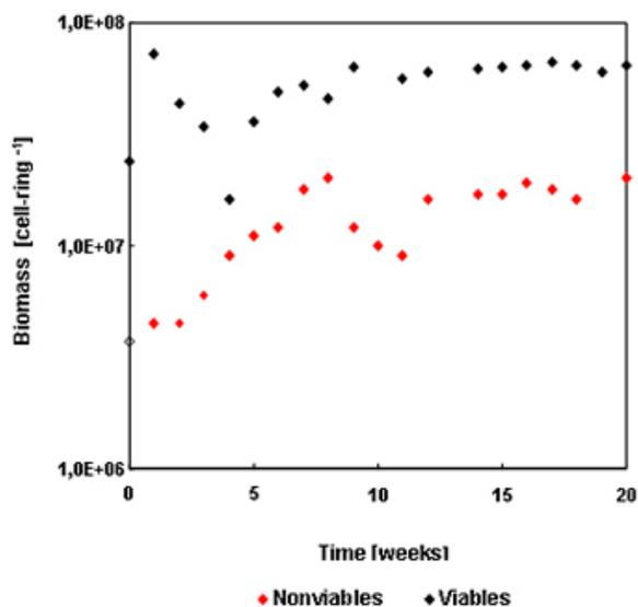
Fig. 2 Cell count in time of *T. thioeparus* on biotrickling filter.
