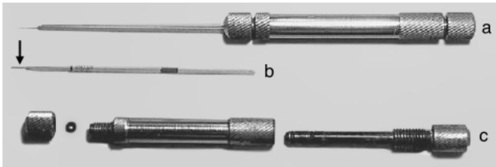
Figure 1. a: Metal piston developed by AEE Soares and JJ Santos (unpublished) used for semen collection from *Apis mellifera* drones' and for instrumental insemination of queens; b: capillary with modified end; c: disassembled metal piston.
