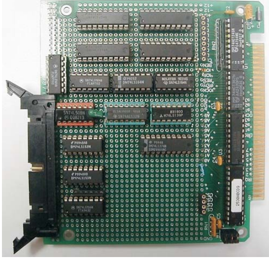
Fig. 8. Acquisition data board tested and working, final design.
