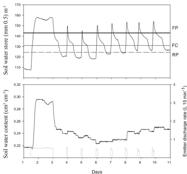
**Figure 2.** Changes in: **A)** the soil water store (SWS) within 0-50 cm depth, and **B)** in the soil water content at the bottom of the active root zone at 50 cm depth). The horizontal lines correspond to the upper limit or “fullpoint” (thick line FP), field capacity (thin line FC) and lower limit or “refillpoint” (dash-dot line RP). The dashed arrows represent the tendency of the soil water store toward field capacity.
