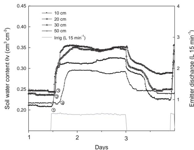
**Figure 1. Changes in soil water content at different depths within the active root zone determined with multisensor capacitance probes during and after an abundant irrigation (0.10, 0.20, 0.30 and 0.50 m). The grey line indicates the emitter discharge rate and the duration of the irrigation event. The numbers within circles indicate the order of detection of the wetted front.**
