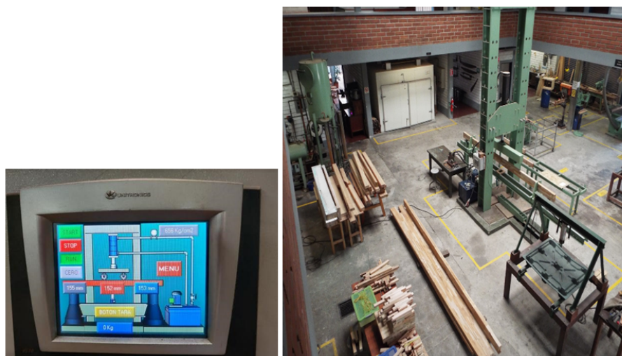
Figure 3. Loading frame capacity 40,000 kg and data processor Unitronics.
