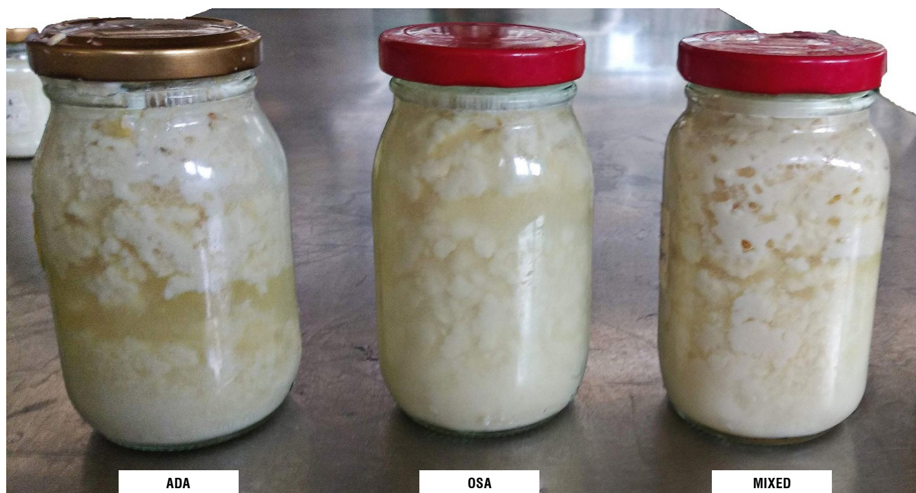
FIGURE 2. Effects of syneresis on treatments with the three types of starch at a concentration of 0.8%: treatments with acetylated distarch adipate (ADA), octenyl succinic anhydride (OSA), and substituted cross-linked starch (mixed).
