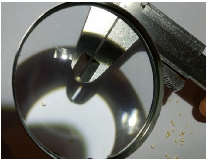
FIGURE 1. Length, width, and thickness measurements of the quinoa grain.
