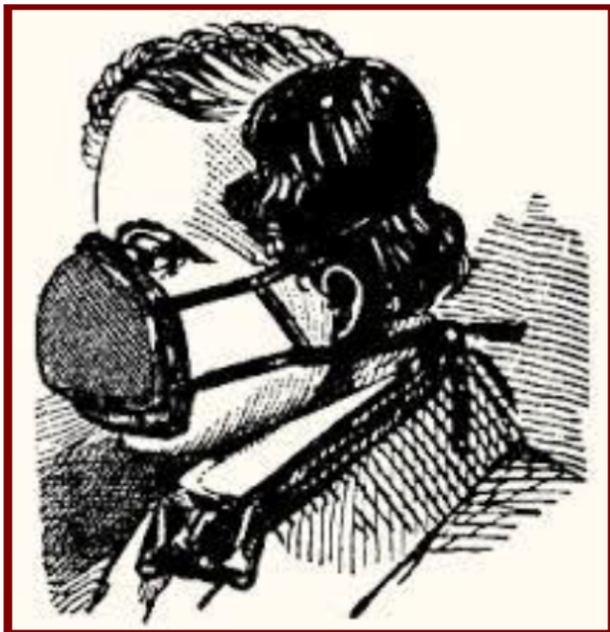
Figure 2 Stenhouse's gas mask.
