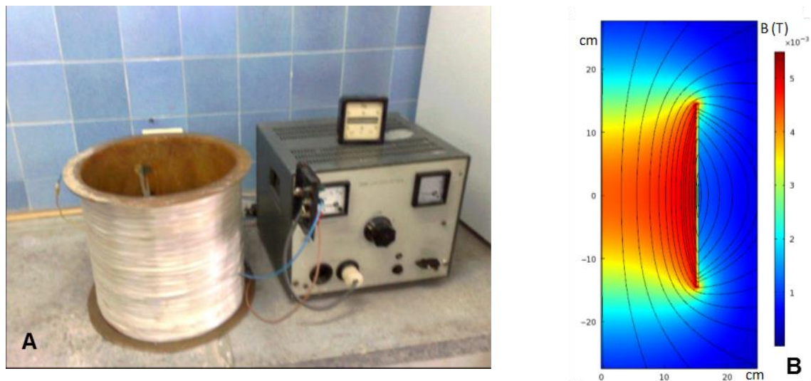
Fig. 1. Experimental equipment of OMF-ELF of 60 Hz. a) solenoid-type coil with air core; b) module surface and magnetic induction lines
