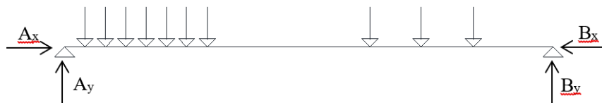
Figure 5: Outline of a beam with four unknowns
