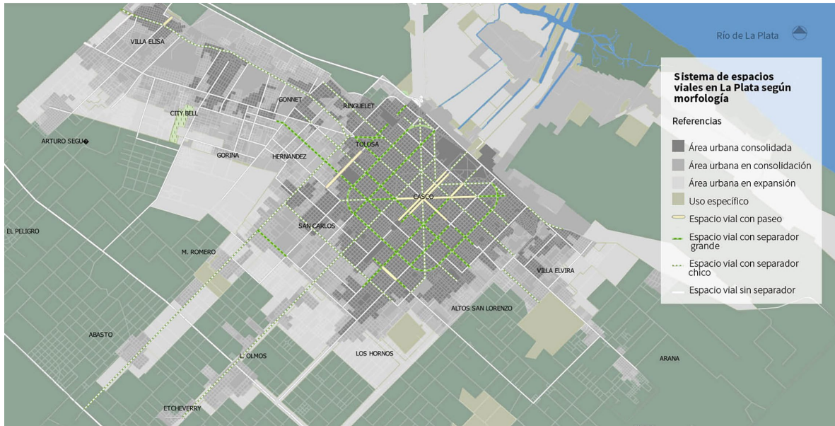
Figure 8. Types of street space by profile in La Plata. Source: Preparation by the Author (2019).
