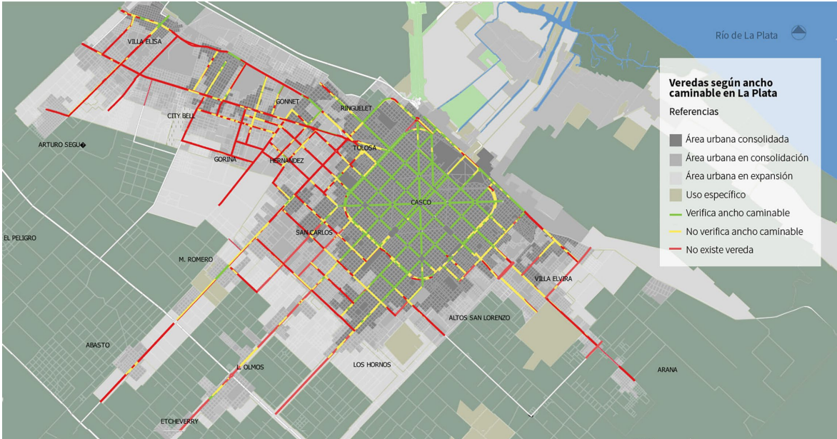
Figure 6. Verification of sidewalks by walkable width for La Plata. Source: Preparation by the Author (2019).
