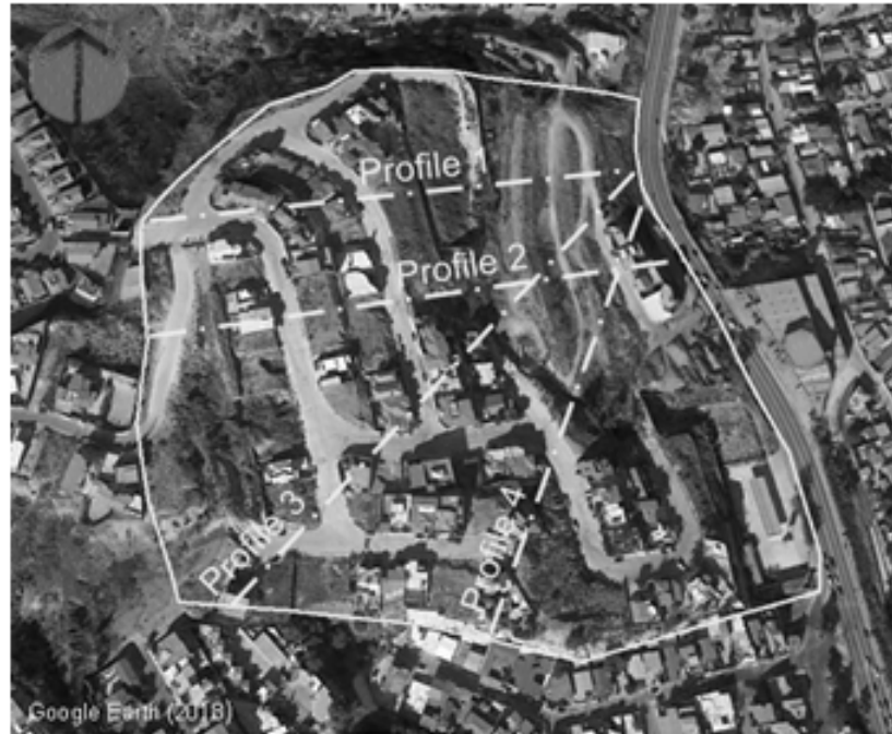
Figure 6. Profiles used for slope stability analysis.
