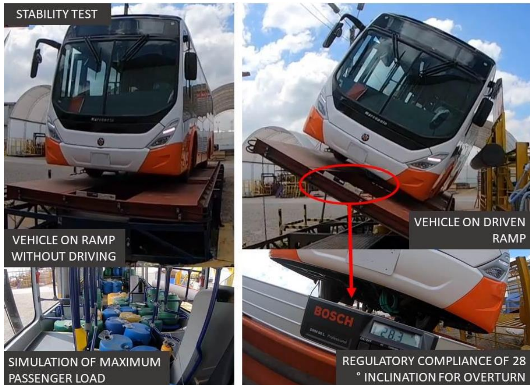
Figure 8. Platform for stability testing. Source: own elaboration
