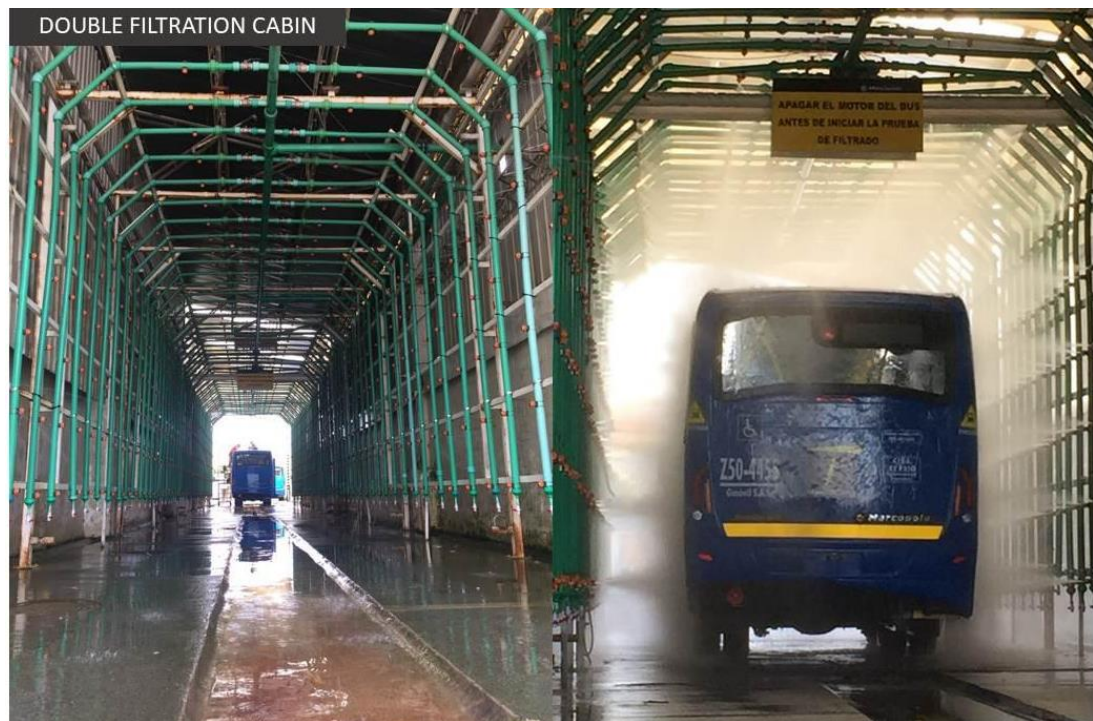
Figure 9. Leak test. Source: own elaboration
