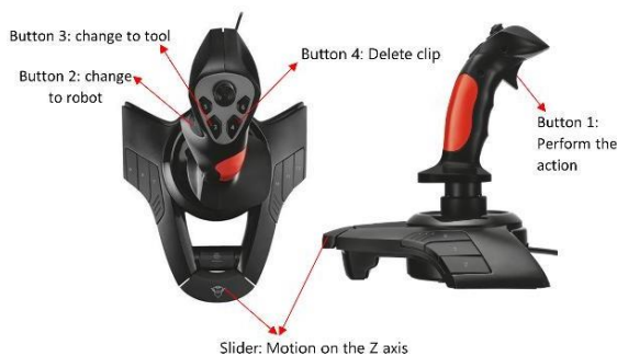
Figure 3. Control actions from joystick. Source: authors
