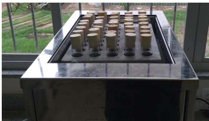
Figure 1. Conventional heating system of incubation tubes in a thermostatic bath at 39°C with manual agitation every two hours, using Tilley and Terry (1963) method.
