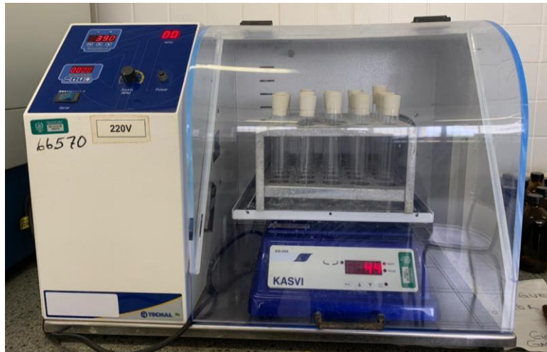
Figure 2. Alternative heating system of incubation tubes in an oven with a temperature controlled at 39°C and constant mechanical stirring at 44 rpm, using the Tilley and Terry (1963) method.
