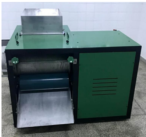
Figure 1. Pulping machine developed to obtain MSM from discarded tilapia carcasses after filleting in a public market in Teresina, Piauí.
