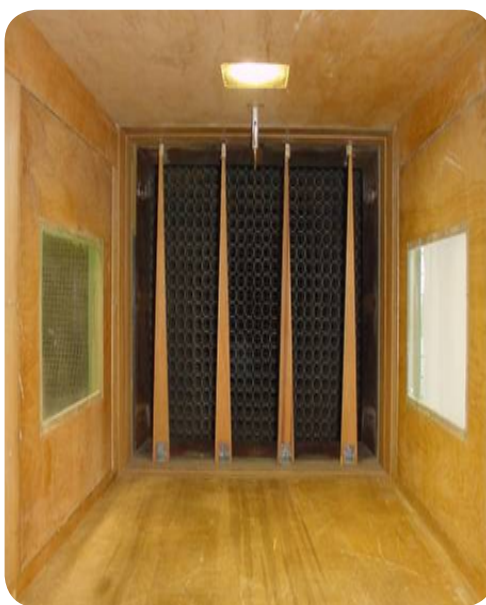
Figure 3. Entrance of the wind tunnel and the turbulence generator.
