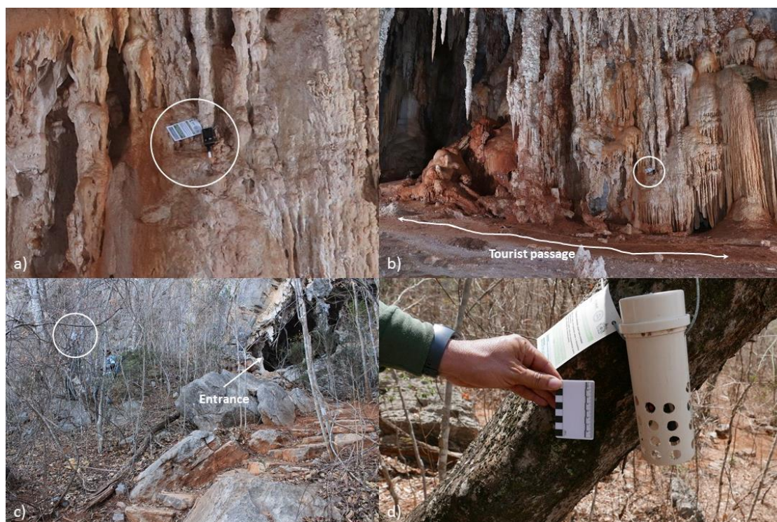
Figure 2 - Installation of the measuring stations in Lapa Bonita. a) Attachment of the equipment on a speleothem, b) Meter installed close to the place of tourist passage, c) Attachment of the equipment on a tree close to the cave entrance, d) Meteorological shelter installed for the external meter.
