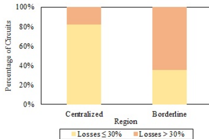
Fig. 4. Percentage of circuits by loss rate range categorized by region.
