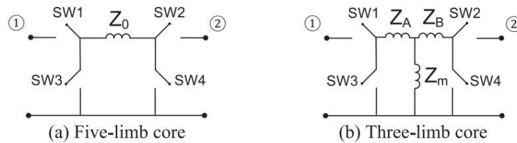
Fig. 4. General series and shunt switch models for the zero-sequence circuit of two-winding transformer, a) Five-limb core, b) Three-limb core [11]
