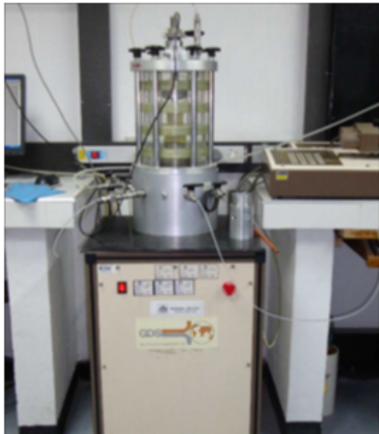
Figure 5 Mechanic devices: a) triaxial testing apparatus; b) compression tester machine Source: Created by the authors
