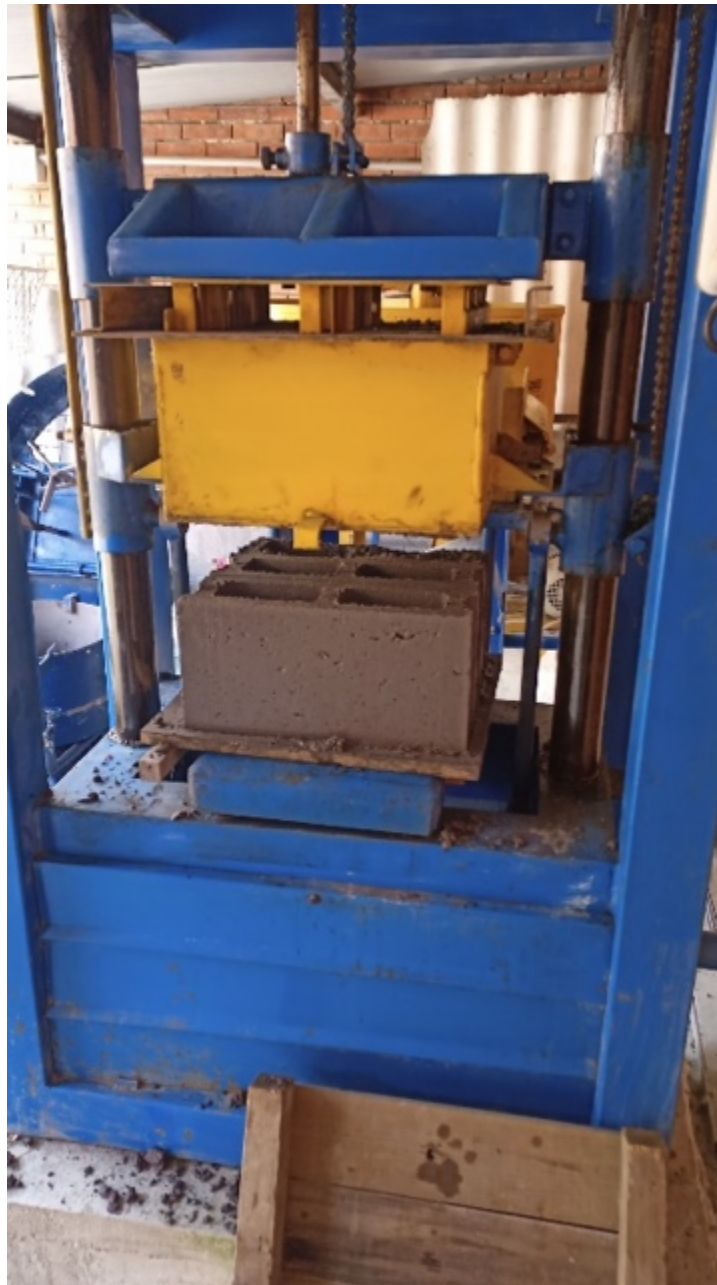
Figure 7. Blocks released from the vibro-compactor Source: own work.
