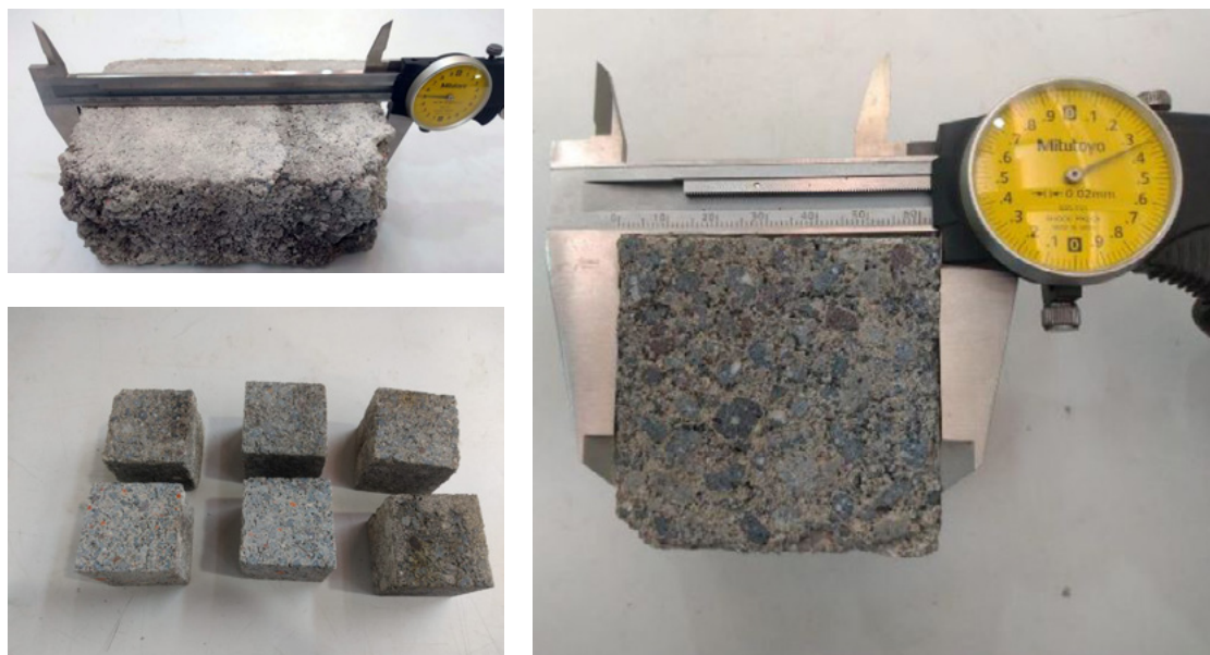
FIGURE 4. Three images showing the preparation process of the piece, in 2020. To acquire the compressive strength, a load was applied at a constant speed and parallel to the longitudinal direction of the specimen, recording the maximum load at failure (Fult), like what has been done by other researchers (Photographs: Alejandro Leal & Alberto Muciño, 2021; source: Authors' Collection).
