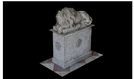
FIGURE 7. Image of the textured mesh in the Escalinata de los Leones , Alcazar of the MNH. 3D model elaborated by digital photogrammetry (Survey and model elaboration: María Sánchez Vega, January 16, 2023; courtesy: Museo Nacional de Historia, CNMH).
