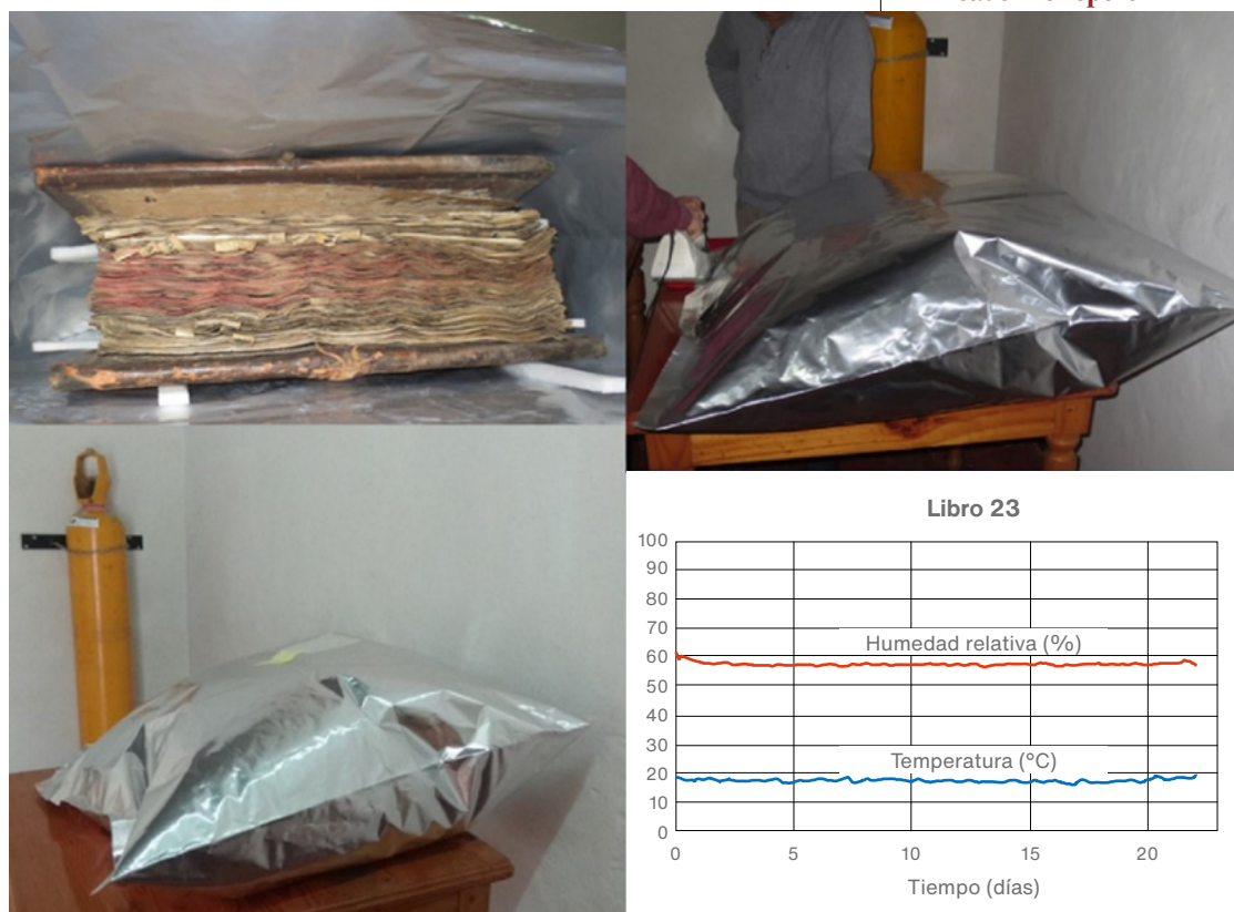
FIGURE 4. Anoxic treatment of Book 23: heat sealing of a nitrogen-filled bag, humidity and temperature monitoring during treatment (Photographs: Javier Nakamatsu, Jhonatan Arízaga, Ivon Canseco, and Patricia Gonzales; courtesy: Museo del Convento de los Descalzos ).
