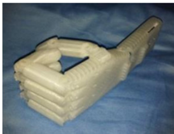
Fig. 2. Mechanical hand prosthesis materialized by additive manufacturing.
