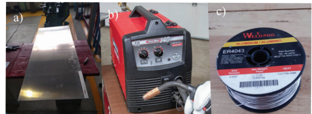
Figure 1. a) 6063-T6 Aluminum sheet, b) MIG welding machine and c) Filler metal ER4043
