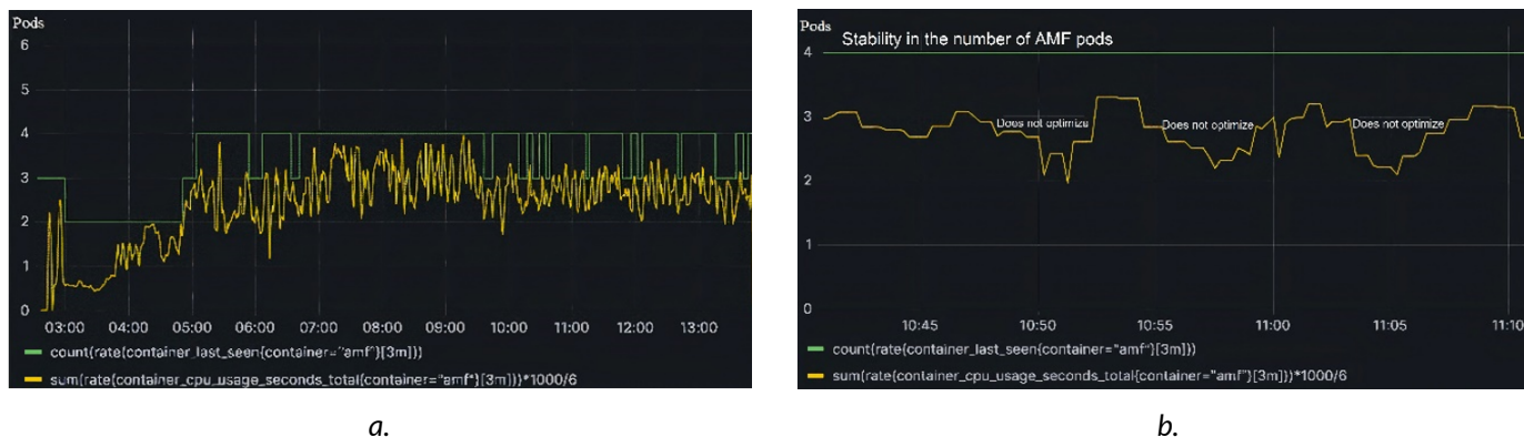
Figure 17. (a) Total CPU usage vs number of AMF pods with 6 mcs threshold; (b) Stability of the number of AMF pods in the face of variations in CPU usage. Self-scaling policies scenario.
