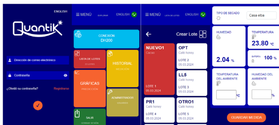
Fig. 4. Mobile app interface of the IoT for analyzing the coffee drying process. From left to right, the main interface, main menu, measurement interface, and measurement recording.
