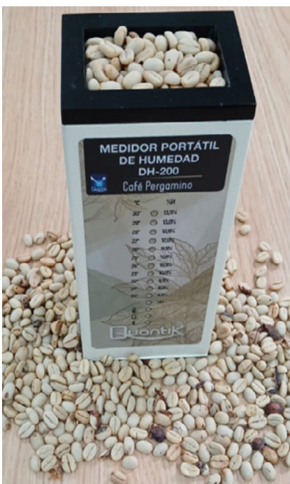
Fig. 2. Portable coffee moisture meter DH-200.
