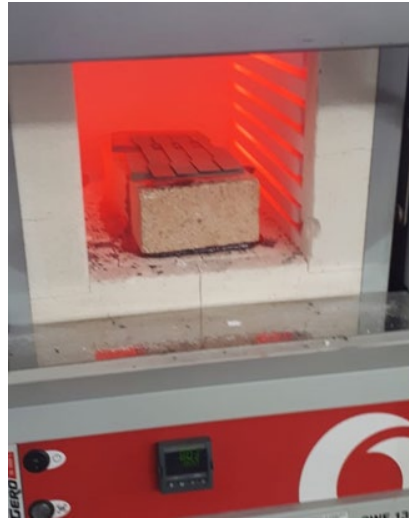
Figure 2. Annealing process of the TRIP and DP specimens. Source: Authors' own elaboration.
