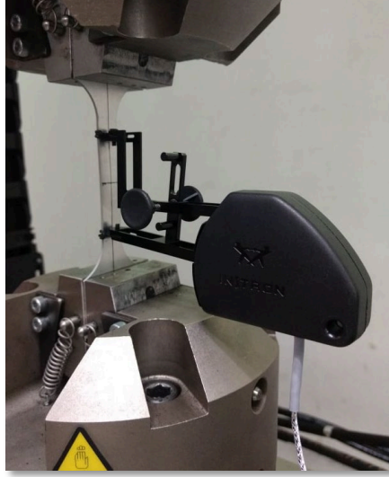
Figure 3. Experimental setup of the uniaxial tensile test. Source: Authors' own elaboration.
