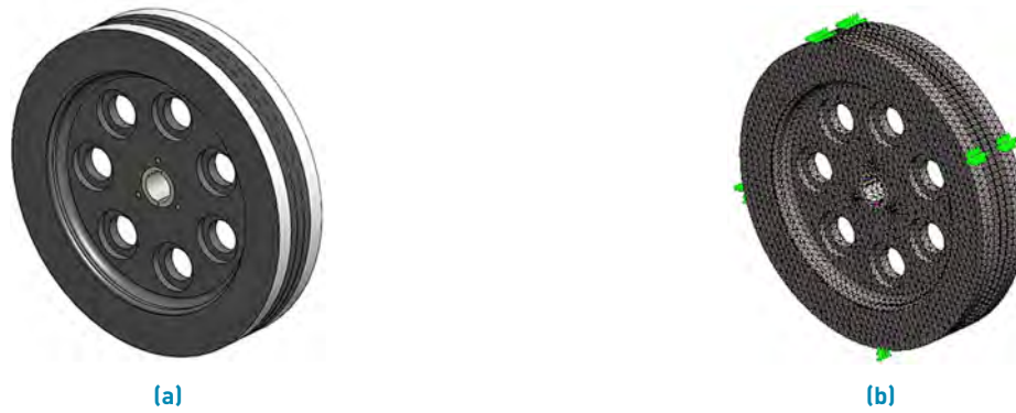
Figure 9 Flywheel: (a) CAD model, (b) mesh, application of restrictions and torque
