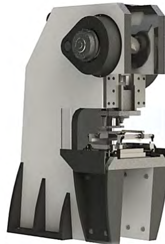
Figure 28 Mechanical test press: rendering and final assembly
