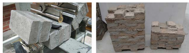
Figure 11 Failure mode of beams under flexural bending: a) prisms with CG blocks, b) prisms with NG blocks
