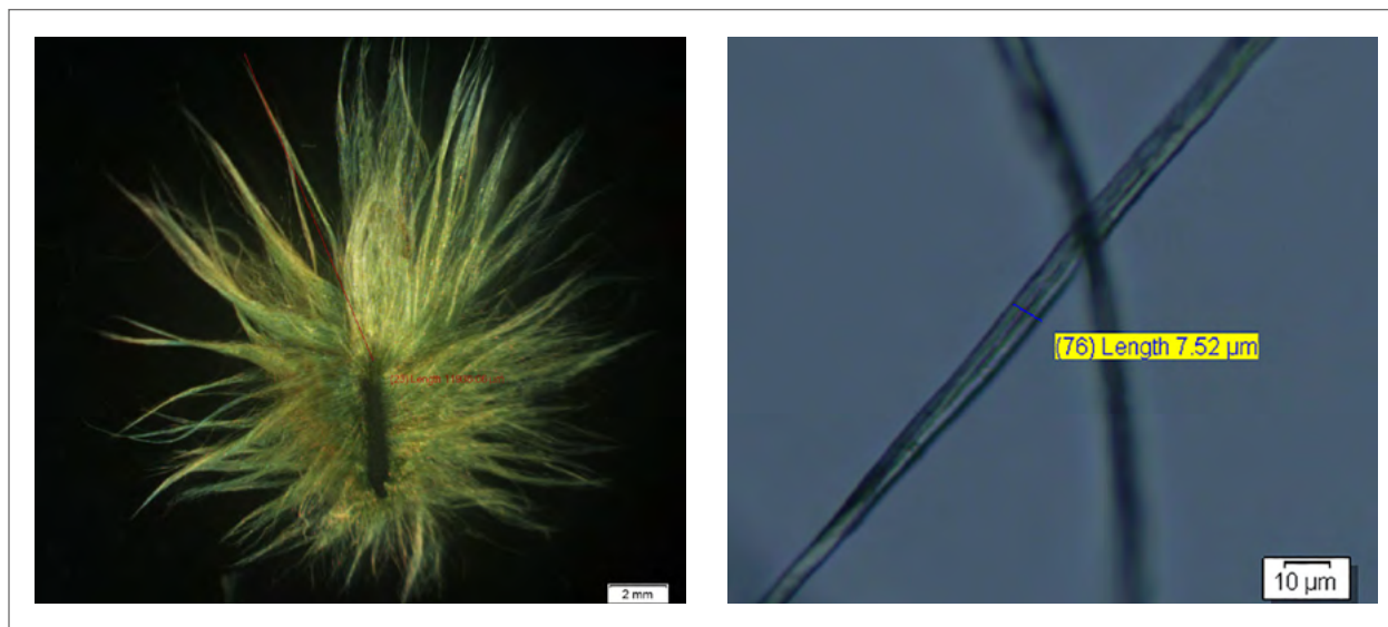
Figure 2. Length and width measurement of the fiber of the wild cotton ecotype ( G. raimondii ).
