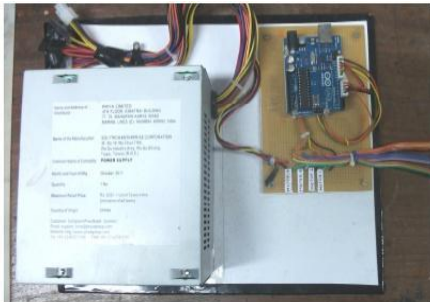
Figure 13. SMPS with arduino uno controller.
