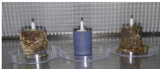
Fig. 2. Air diffusers at the end of removal test No. 2. From left to right: Aspergillus sp., control, and Penicillium dipodomyicola strain IIF7SW-F4.
