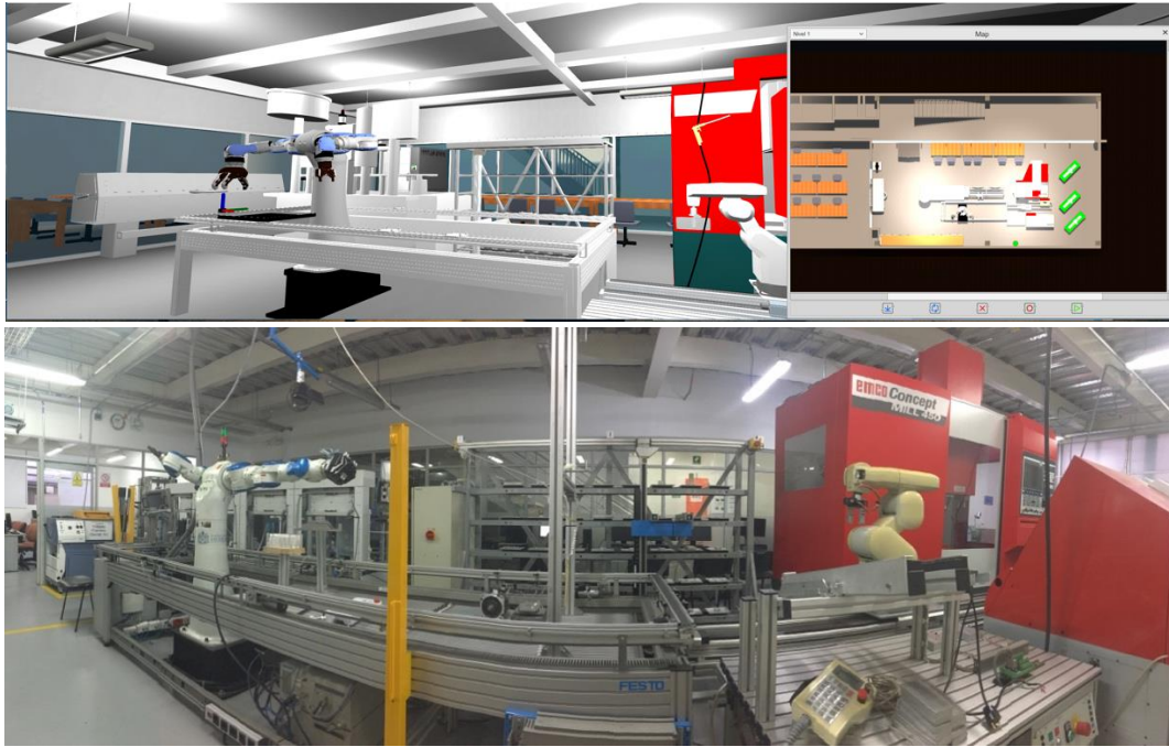
Figure 13. Snapshots of the CIM training game based on BIM. Comparison between real CIM and the virtual world
