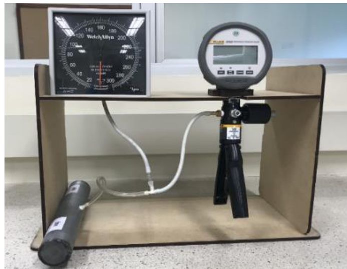
Figure 2. Sphygmomanometer calibration setup
