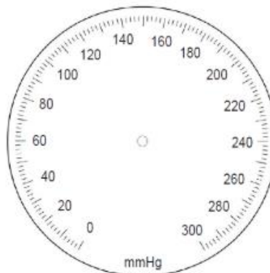
Figure 1. Example of a manometer aneroid scale (divided in mmHg without a zero-tolerance zone)
