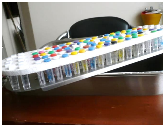
Fig. 1: Individual containers specially designed to hold samples in distilled water at 37 °C.
