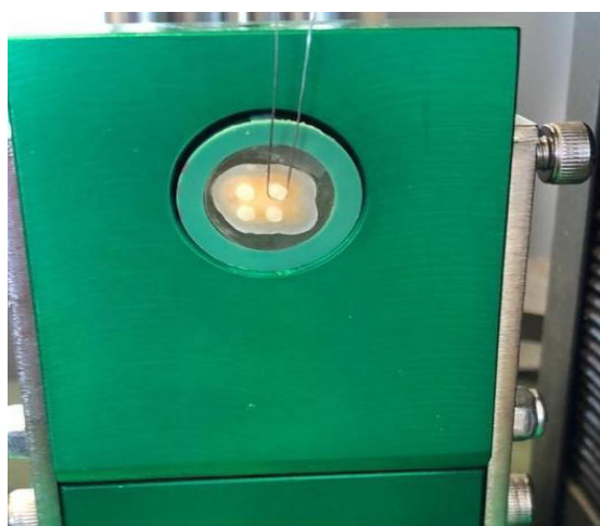
Fig. 2: Universal testing machine performing micro-shear mechanical test.
