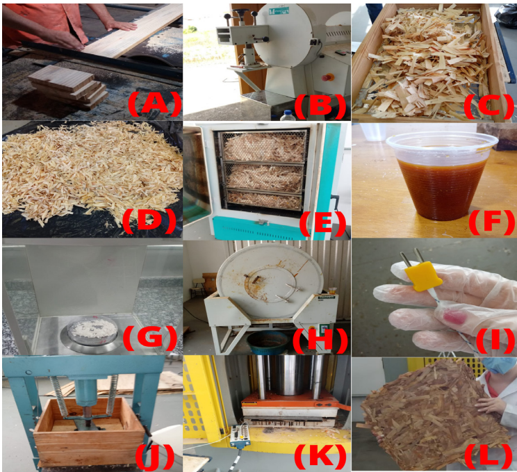
Figure 1: Production process of the boards. (a) Wood processing; (b) Wood chipping; (c) Strands classification with 5 mesh shive; (d) Natural drying of the strands; (e) Oven drying; (f) Preparation of the adhesive; (g) Weighing of nanoparticles (h) Mixer-rotating drum; (i) Thermocouple type K; (j) Pre-pressing; (k) Hot pressing; (l) Finished panel.
