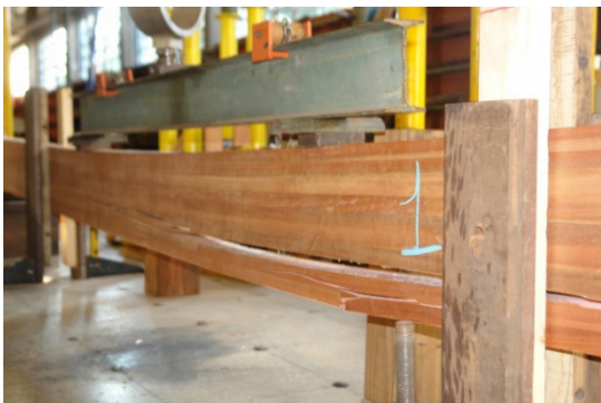
Figure 7: Detachment by shear due to unsatisfactory adhesion.
