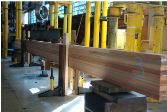
Figure 3: Test set-up of four-point bending test.
