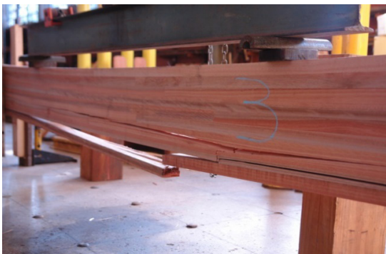
Figure 6: Failure mode started in the finger-joint.
