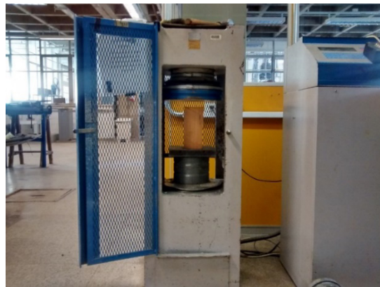
Figure 4: Test set-up of compression parallel to the grain test.
