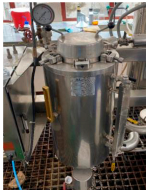
Figure 3: Autoclave used for the water impregnation.
