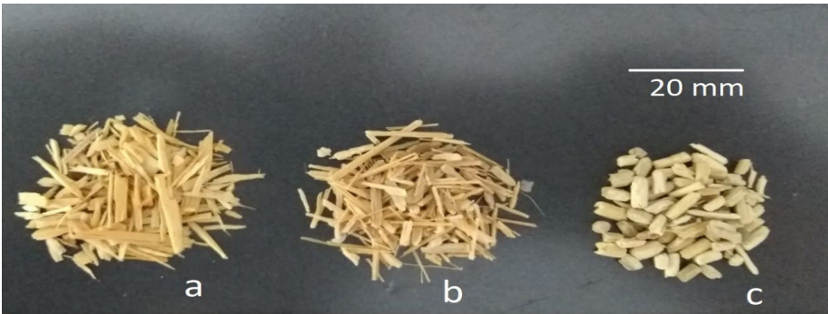
Figure 2: Particles commercial (a) Pinus taeda , (b) Bamboo and (c) Mate produced in the laboratory.
