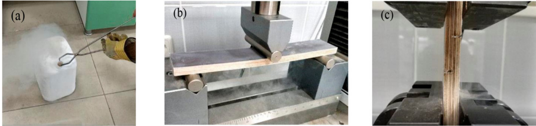
Figure 1: (a) Freezing treatment of plywood samples, (b) bending test, (c) tensile-shear test.
