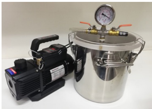
Figure 4: Saturation was reached in approximately 60 min compared to several days submersion without vacuum support.
