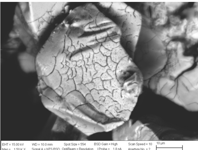
Figure 8. SEM image from the leaching residue of the -53+38 \mu\text{m} particle size concentrate pre-treated with 15% of HCl. Source: The Authors
