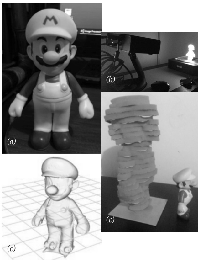
Figure 7. a) Real object, b) object in scanning process, c) digital object, d) object reproduced in foam.
