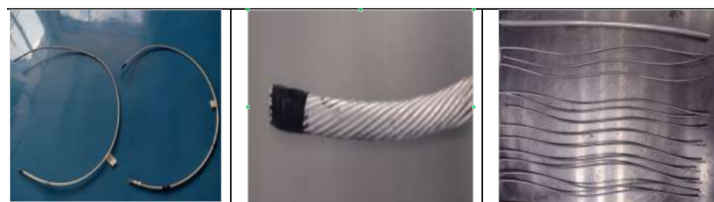
Figure 8. 0.30 m long OPGW cable for tension tests, aluminum tube containing the optical fibers and their 12 test wires
