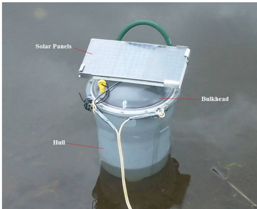
FIGURE 8 Buoy station prototype field test.
