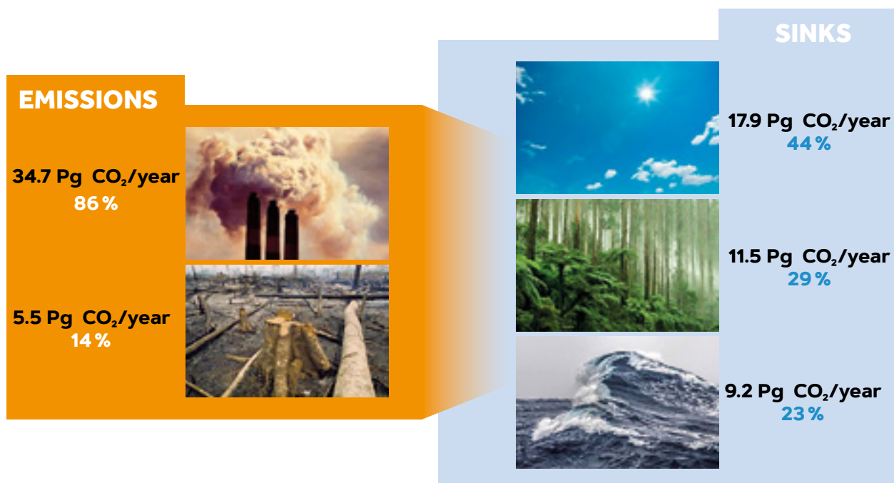
Figure 2. Annual CO 2 emissions (average for the period 2009–2018) derived from the burning of fossil fuels and deforestation, and the three compartments that act as CO 2 sinks: the atmosphere, ground vegetation, and oceans.
